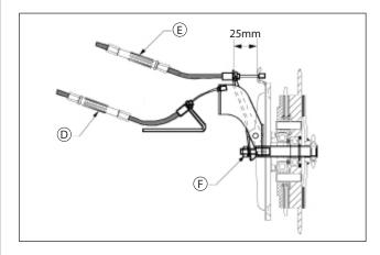
The roller clutch can be adjusted, with the cable inline adjuster and also by the locknut fitted to the pull rod
