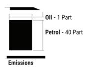
The engine uses two-stroke fuel. If you have emission requirements, the mixture ratio of the fuel to oil should be 40:1.
