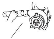
Connect blower tube to unit by rotating it into place. Interlock blower tubes together with the same rotation motion.
