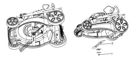
NOTE: Be sure to replace the parts in the exact order in which they were removed. When installing the cutting blade, verify that it is installed with the curved ends pointing toward the mower deck, and not toward the ground.
